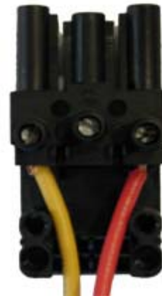
(6B) Jumper Wire Removed, Remote Timer used in conjunction with on board timer.
